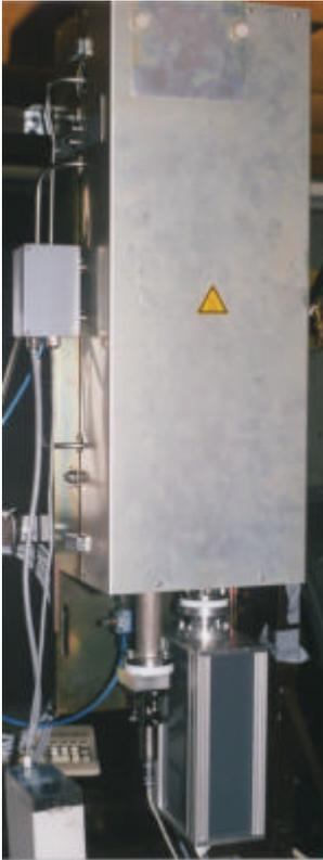
The measurement cell and the exhaust gas tubes are heated and thermo-controlled to avoid conflicts with deposition and interferences by condensation i.e. formation of water droplets.
