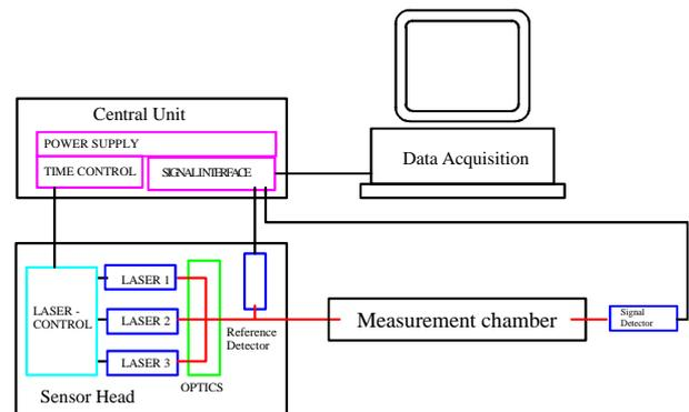
Fig 1: Schematic of the new sensor
