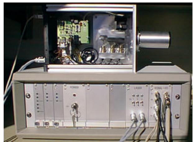
Fig. 2: Sensor head with supply and interface unit
